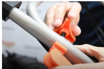
3. Fix the cables with the clamps .
