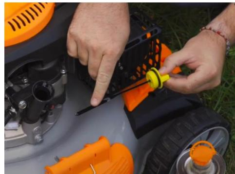
Change the engine oil after the first 5 hours of operation, which is the break-in period, then every 25 hours of operation or every 6 months.
