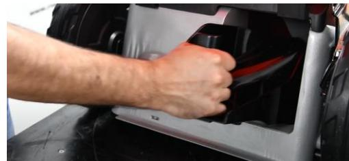
3. Place the starter rope on the support hook.
